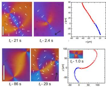
a) Aligned defect pair in homogenous director field. The black arrow is the outer director field orientation. b) Misaligned defect pair. The final annihilation orientation is perpendicular to the outer director field.
