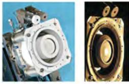
HETs : (a) PPS-1350 and (b) PPS-1350 severely eroded (Credits Safran)
