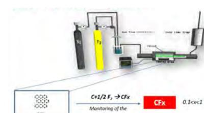
Graphite is placed in a furnace under vacuum. F<sub>2</sub> gas is injected in the furnace and **temperature** is increased
