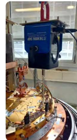
Fig 3. mini shaker attached to cryostat cold plate for hot vibration testing
