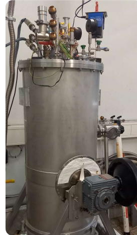
Fig 2. helium bath cryostat for the study of the dissipation induced by microvibrations
