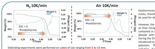
Debinding experiments were performed on cubes of size ranging from 5 to 15 mm. Based on the TGA under  $N_2$  a debinding profile was built, with significant improvements compared to the industrial cycle achieving a critical wall-thickness of 7 mm, compared to a critical wall-thickness of 5 mm before. Exothermicity promotes the creation of cracks, therefore a **nitrogen atmosphere** will be used for debinding experiments.
