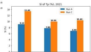
Fig. 2 : Validation of Peak period (Tp) in MFWAM simulations in 2021 with SPOFAR (SPOTTER) buoys
