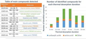
The first results indicate that a maximum of compounds are extracted between 5 and 7.5 min of thermal desorption.
