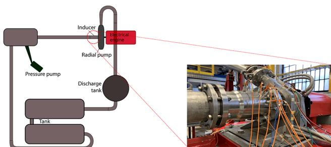
Quantification of **radial efforts** on the shaft's turbopump
