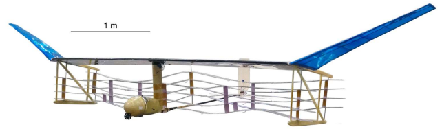
Fig. 2: Xu, Nature 2018 [2] Prototype of a model aeroplane powered by an ionic wind thruster.
