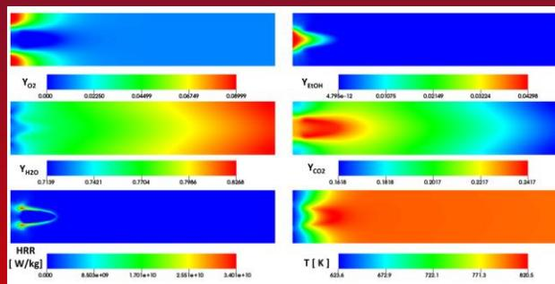
Contour plots for  $T_{injection} = 350\text{ C}$ ,  $U = 10\text{ mm/s}$  (both fuel and oxidizer) (Simulation done using NOTUS on supercomputer of CNES)
