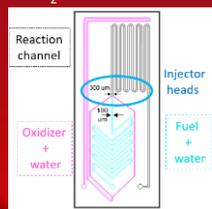
Injector head to facilitate premixing.
