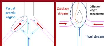
Premixing of fuel and oxidizer
