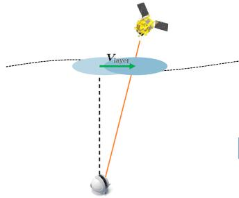
Predictive controller accounts for evolution during delay. In LEO-to-ground case, information of apparent wind speed **known from orbit**.
