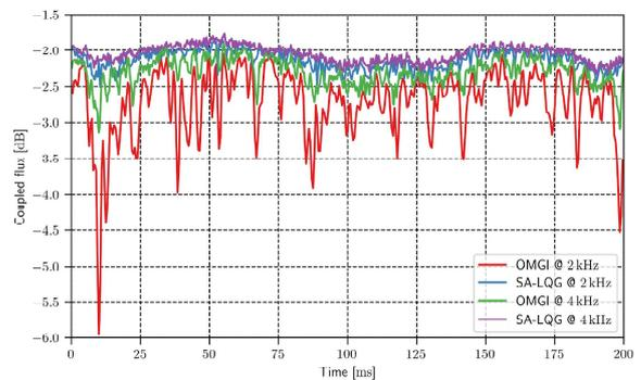
Predictive controller (SA-LQG) vs. classical integrator (OMGI). Use of two different loop frequencies.
